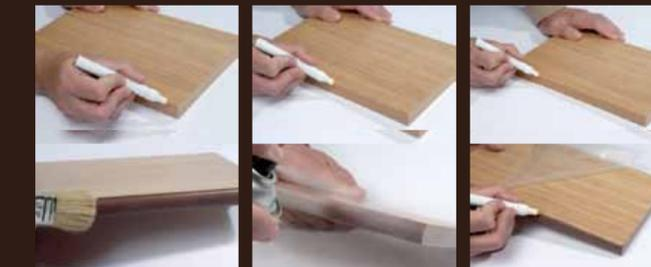
2. Or perhaps, if you want to chamfer up the edge leaving the MDF raw. This is perfectly possible. You can then finish it with a water-based lacquer which you can apply with a spray gun or a brush. (the polythene film is there to protect the face). This being done, you use the same technique as in the previous case: you peel off the film and you finish the tiny corner with a light sanding followed by the stylo pen.
